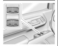
The power windows work when the ignition is on, in acc/accessory, or when Retained Accessory Power (RAP) is active. See Retained Accessory Power (RAP)
