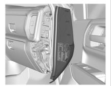
The right instrument panel fuse block access door is on the passenger side edge of the instrument panel.
