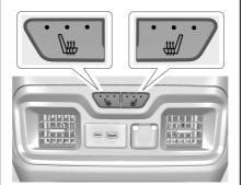
If available, the buttons are on the rear of the center console. To operate, the engine must be running.
