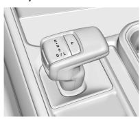
The shift pattern is displayed on the top of the shift lever. The selected gear position illuminates red on the shift lever, while all others will be displayed in white. If the shift is not immediate, as in very cold conditions, the indicator on the shift switch may blink until it is fully engaged. The shift lever always starts from a center position, represented by an up/down arrow on the shift pattern. After releasing the shift lever, it will return to the center position.
