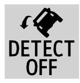
If equipped, the rollover detection disable button will be on the center stack in either the first, second, or third position.
