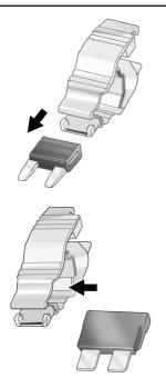
3. Use the fuse puller to remove the fuse from the top or side, as shown above.
