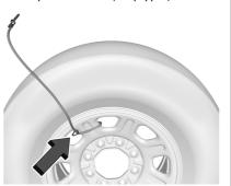
If equipped with a spare tire cable, reinstall the cable to the spare wheel by looping the cable around a wheel vent window then pass the clip end of the
