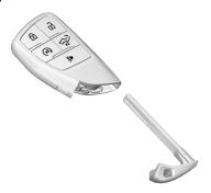
Press the button to remove the key. Never pull the key out without pressing the button.
