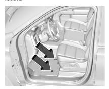
Reinstall by lining up the floor mat/liner retainer openings over the carpet retainers and snapping into position.
