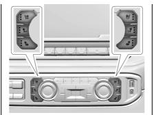
Heated and Ventilated Seat Buttons Shown, Heated Seat Buttons Similar
