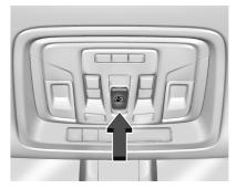
If equipped, the power sliding rear window works when the ignition has been turned on or to accessory mode, or Retained Accessory Power (RAP) must be active. See Retained Accessory Power (RAP) ⇒ 219.
