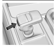
This vehicle is equipped with an electronically controlled transmission. The shift lock release button is designed to prevent inadvertent shifting out of P (Park) unless the ignition is on, the brake pedal is applied, and the shift lock release button is pressed.
