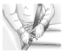
To unlatch the belt, push the release pushbutton on the buckle. The belt should return to its stowed position.
