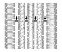
Treadwear indicators are one way to tell when it is time for new tires. Treadwear indicators appear when the tires have only 1.6 mm (1/16 in) or less of tread remaining. See *Tire Inspection* ⇒ 349 and *Tire Rotation* ⇒ 350.
