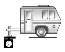
Do not exceed a maximum trailer tongue weight of 567 kg (1,250 lb) for a conventional trailer hitch.
