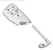
Remove the key by pressing the button on the side of the remote key near the bottom and pull the key out. Never pull the key out without pressing the button.
