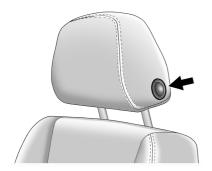
To raise or lower the head restraint, press the button on the side of the head restraint and pull up or push the head restraint down and release the button.
