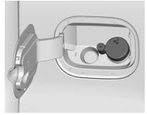
The vehicle has a locking fuel fill cover. Use the fuel fill cover key to unlock the cover. The key cannot be removed in the unlocked position. When reinstalling the fuel fill cover, be sure the arrow is pointing straight up.
