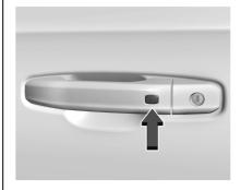
If equipped, the remote key must be within 1 m (3 ft) of the tailgate or door being opened or locked. Press the button on the door handle to open. See "Keyless Access Operation" in *Remote Key Operation*
