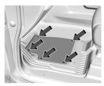
Reinstall by lining up the floor liner insert button clips over the liner retainers and snapping into position.
