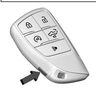
If the vehicle has the Keyless Access system, the remote key has a button on the side of the remote key used to remove the key.
