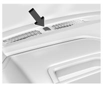
The indicator light, on the instrument panel near the windshield, indicates the status of the system.
