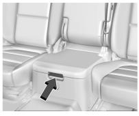
If equipped with front center seat storage, unlock with the mechanical key in the remote key, press the latch, and lift to open.
